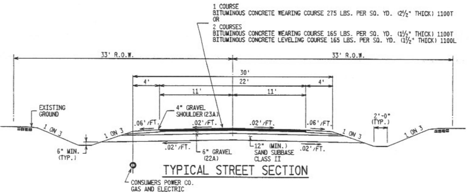
NOTE: Any ditch which is not a part of a county drain system shall have a 1 on 3 slope front and back. All others shall be as directed by the Midand County Drain Commission.
